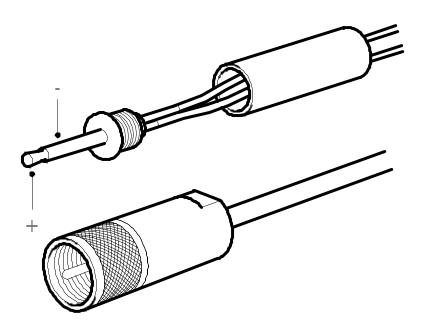
Use an ohmmeter to determine which of the terminals is the (+) and (-) of the jack plug.
