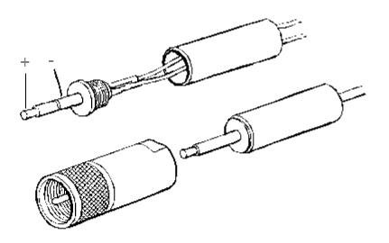
Use an ohmmeter to determine which of the terminals is the (+) and (-) of the jack plug.
