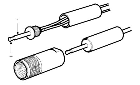
Use an ohmmeter to determine which of the terminals is the (+) and (-) of the jack plug.
